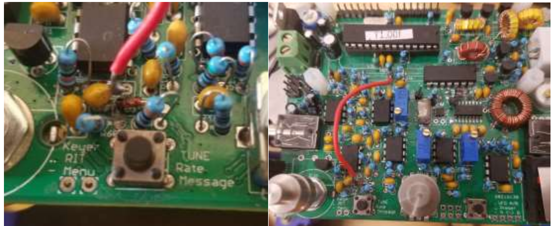
Figure 53: C20 with one end connected to PCB and the wire attached to lead (left) and completed modification (right)
