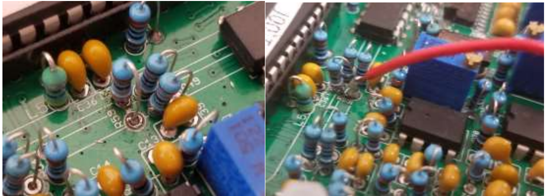
Figure 52: R59 with orientation changed (left) and jumper attached (right)
